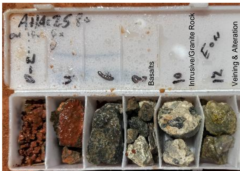
Chip tray, AHAC1258, February 2025 AC hole, Basalts, Intrusives, Alteration and veining visible, Assays Pending
